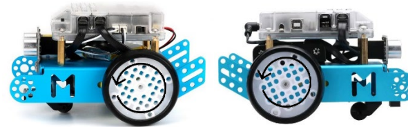
Figure 9. Direction of Motor Rotation in the mBot2.
